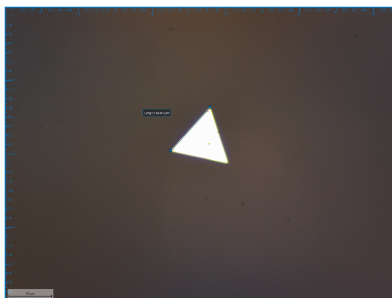
Figure 10: Optical Microscope Image of a Triangular Flake Fabricated with Supersaturation Monitoring
